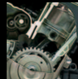
New cylinder block - Features sleeveless JCP (Jet-flow Circulation Plating) cylinder walls for lighter weight, minimised friction and tighter spacing of larger-bore cylinders.
