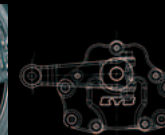
New HESD - Smaller, lighter-weight new second-generation Honda Electronic Steering Damper located behind steering head enhances high-speed and cornering control.
