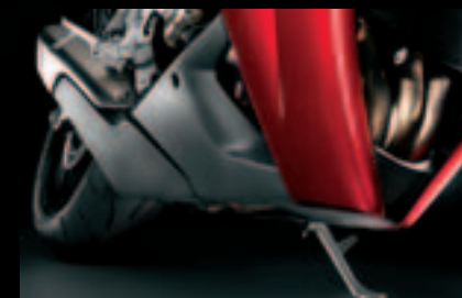
New underbelly exhaust - Concentrates weight and mass under the engine for lighter, more responsive steering control. Short upswept tailpipe shaped for maximum cornering clearance.
