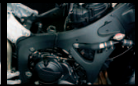
Die-cast aluminium frame - Lightweight, mass-centralising FDC (Fine Die-Cast) aluminium frame is precision moulded in a strong, slim and compact configuration that delivers responsive handling and world-class racing potential.
